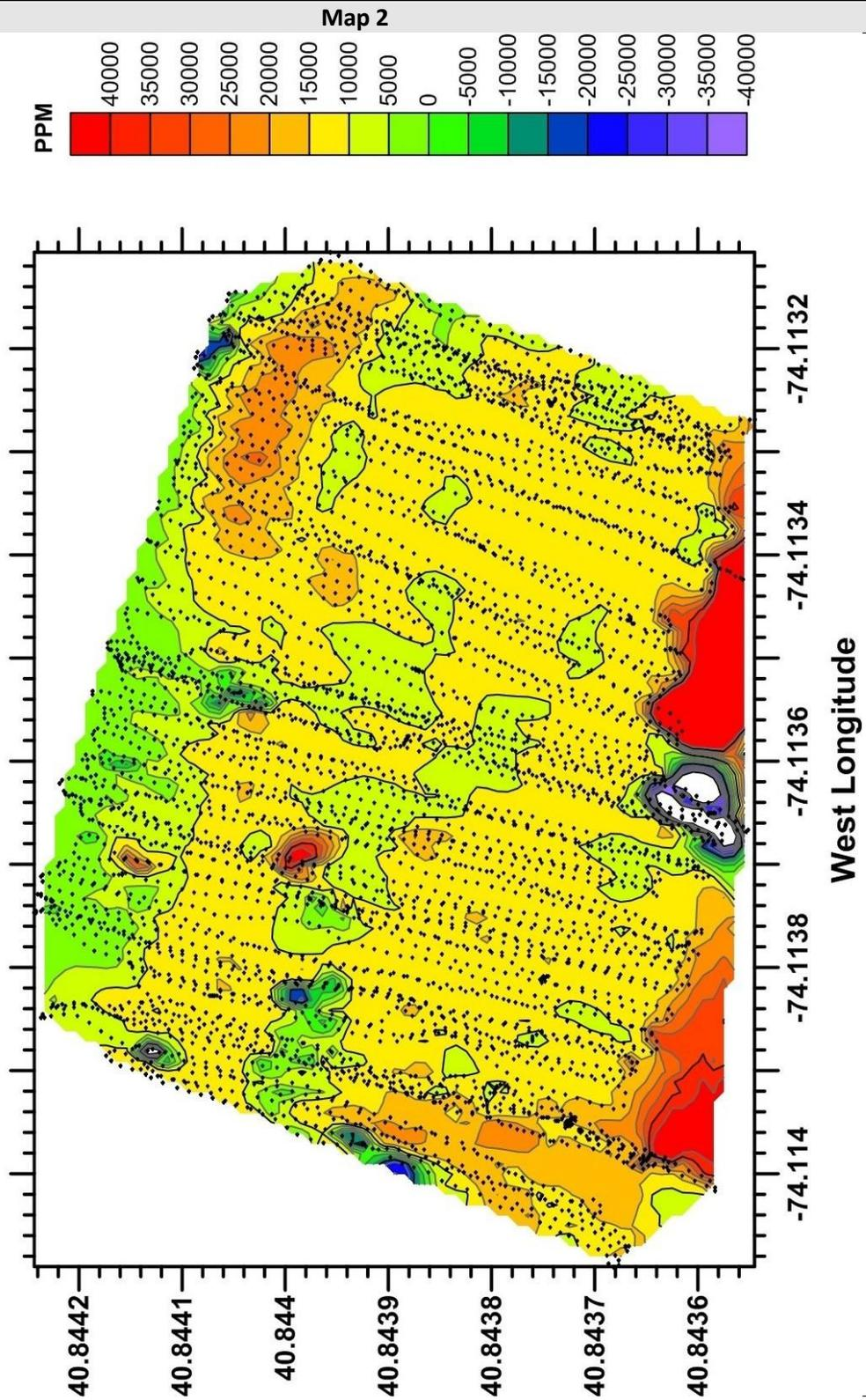
In-Phase electromagnetic induction data for the 8KHz frequency. This is a horizontal slice corresponding to a depth of around 1-2 meters.
